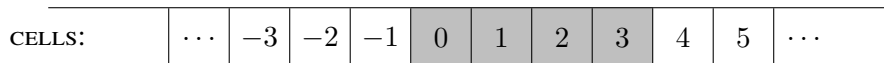
Figure 3.1: Numbering of tape cells of a one-tape Turing machine. The shaded part is a potential input of length 4.
